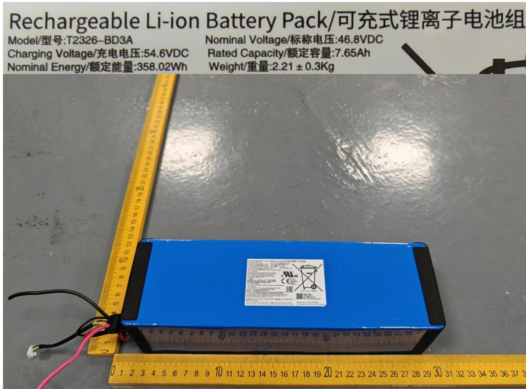
Battery / 电池组 (T2326-BD3A 46.8V 7.65Ah 358.02Wh)
