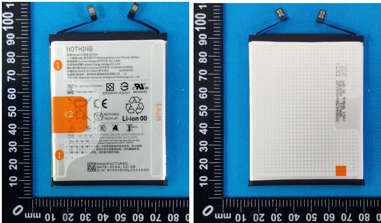
Single Cell Battery /单电芯电池 (NT05A 3,86V 5150mAh 19,88Wh)
